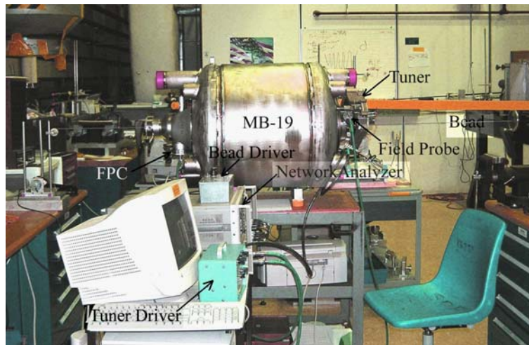
Figure 4: Bead-pulling setup to measure the field flatness of SNS MB-19 with Helium Vessel.
