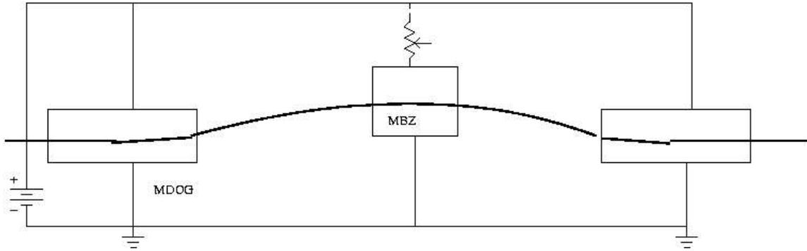
Figure 2: Relationship between magnets, power supplies and shunts in doglegs 5 through 9.
